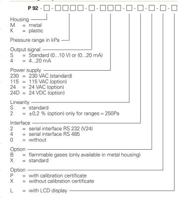
**Example:** Sensor in a metal housing with measurement range 1.0 kPa; output signal 4...20 mA; power supply 230 VAC; linearity  $\pm 0.5\%$ ; without certificate of linearity; non-flammable gas; without serial interface: P92M-1.0-S-230-S-0-X-X
