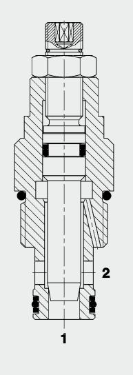
The SD10 is a flow control valve which controls the flow rate by adjusting the cross section. The flow rate is therefore dependent on the pressure differential and viscosity. Starting with the throttle spindle in the fully closed position, the flow rate increases in accordance with the appropriate curve as the control knob is turned. The flow is controlled in
