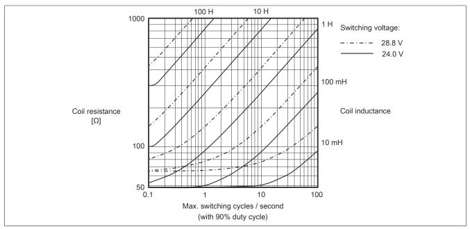
Environmental temperature: 60°C, all outputs with the same load
