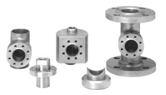
Diaphragm seals are designed to isolate the sensing element of pressure gauges and pressure switches from process fluids which may be corrosive, viscous, sedimentous and/or with a high temperature. The diaphragm is welded to the upper body, to ensure separation of filling fluid from process medium. The "in-line" diaphragm position enables deep cleaning of their surfaces. Flange clamping with metallic sealing guarantees the system against leakage at high process fluid temperatures and pressures.
