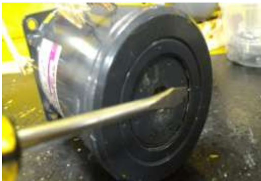
STBD ACTUATOR MOTOR (CRACK AT CASING MOTOR)
