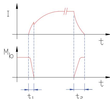
**Note:** The timing of intervention ( $t_1 - t_2$ ) are shown in the tables on pages following while the delay time ( $t_r$ ), since it depends on the inertia of the load and the energy stored by the motor, can not be estimated because it varies from motor to motor.
