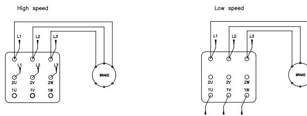
Self-braking three-phase **two-speed** motors - **double winding** - with dc brake
