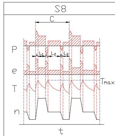
**Duty-type S8:** continuous operation duty with related load/speed changes.
