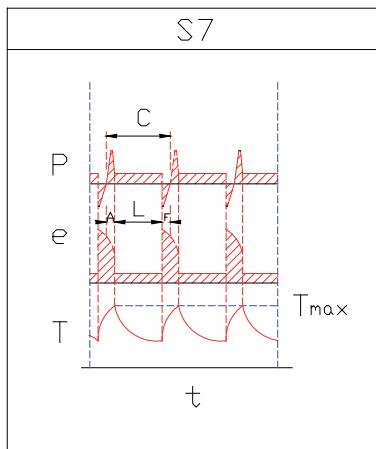
**Duty-type S7:** continuous operation duty with starting and braking.
