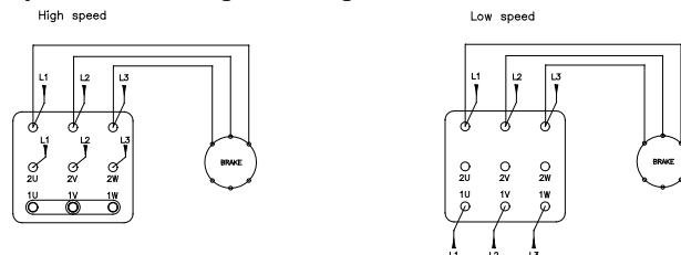
Self-braking three-phase **two-speed** motors - **single winding** - with dc brake
