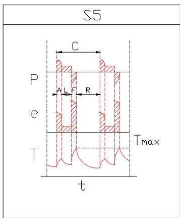
**Duty-type S5:** intermittent periodic duty with electric braking.
