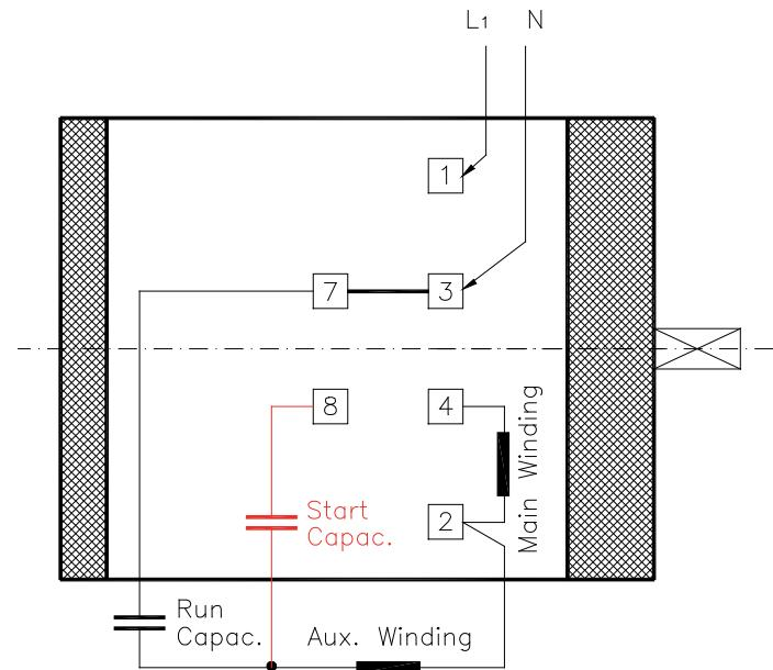
To reverse rotation, interchange the wires of the main winding
