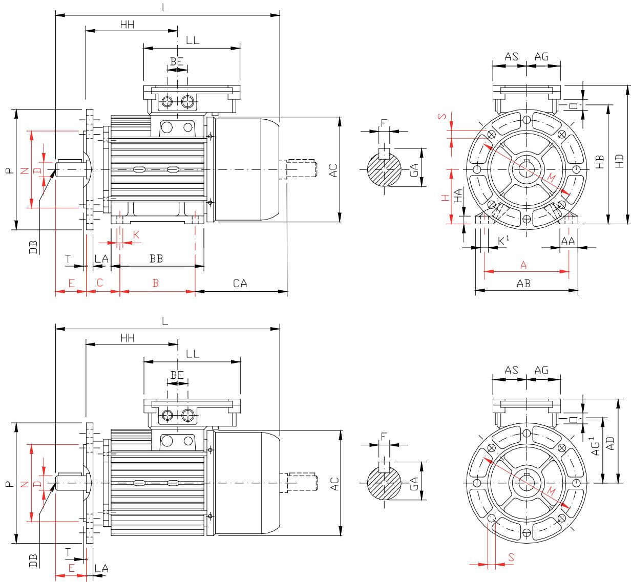
**Note:** Ledge of the second shaft, from size 71 upwards, is reduced to a size.
