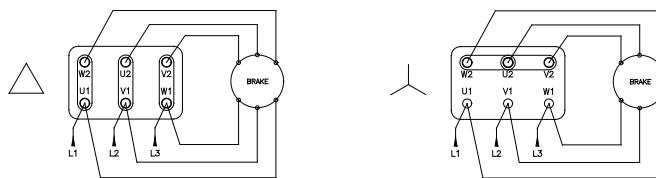
Self-braking three-phase **one-speed** motors - with dc brake
