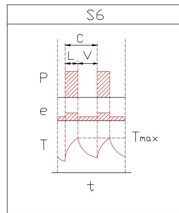
**Duty-type S6:** continuous operation with intermittent load.
