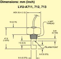
Protection: Transient, reverse polarity Sensor: 316 LSS Temperature: -29 to 80°C (-20 to 176°F) Pressure: Up to 1000 psig (6895 kPa) Mounting: ¼ or ½ NPT (depending on model number)
