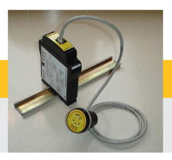
**REMLIVE RL-24i** is the latest addition to the range of **REMLIVE** electrical safety warning products. Its purpose is to provide **CONFIRMATION OF CORRECT ISOLATION**. The **REMLIVE RL-24i** kit comprises two units, one door or flange mounting and one din rail mounting. The door unit is designed to fit through the front of a control panel or switch and occupies a standard 30.5mm pushbutton hole. It is rated at IP 65 for Europe and NEMA 4X for USA.
