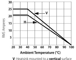
H: Heatsink mounted to a **horizontal** surface.
