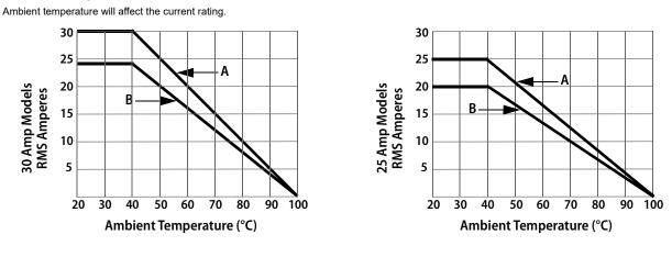
A: Single relay or with 0.75" spacing between relays. Derate above 40 °C; subtract 0.5 amp/°C.
