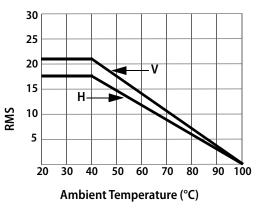
V: Heatsink mounted to a **vertical** surface H: Heatsink mounted to a **horizontal** surface.
