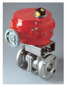
Stem Seals Flanged Series  $^{1}/_{2}$ "-2" valves feature live-loaded, self-adjusting primary and secondary sealing. Utilizing belleville washers, the stem seal automatically adjusts to compensate for changes in temperature and normal wear.  $2^{1}/_{2}$ "- $1^{2}$ " valves utilize an independent packing gland which can be easily adjusted without removing mounting hardware or operator. The packing gland is contoured to more uniformly distribute the load across the packing.
