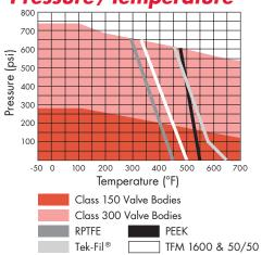
**Note:** Carbon Steel valves limited to -20°F.
