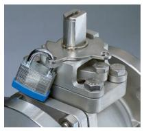
All manually operated valves feature a **Locking Device** to prevent accidental movement of ball position. Valves  $^{1}/_{2}$ "-2" feature a safety trigger that locks the handle in the open or closed position. The handle lock can be bypassed, if needed, with a small bolt through the handle in the release position. On all sizes a **Padlock** can be added to secure the handle in position, preventing unwanted movement of the ball.
