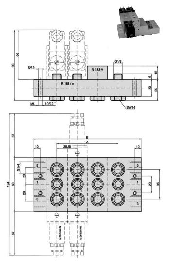
**Dimensions for P-R-S-manifold R-183**
