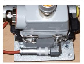
Figure 4: Main connector with heater attached.
