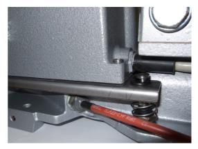
Figure 3: Base plate heating element.
