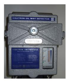
Figure 1: Measuring Head of VN87plus series.
