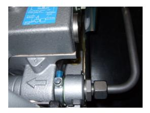
**Figure 8:** Air jet pump with scavenging kit installed (connector ring, seals new venture injector and hose).
