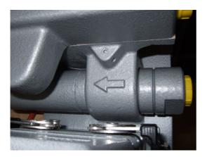
Figure 7: Air jet pump without scavenging air kit.
