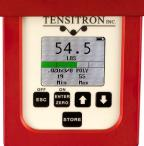
Precise, convenient tension measurement for strapping and tiedowns.
