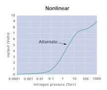
Standard analog output is 0 to 7 Volts that is linear in voltage with the log of pressure. Two alternate analog outputs can be selected using the front panel buttons: either 1 to 8 Volts that is linear in voltage with the log of pressure or 0 to 9 Volts that is non-linear with the log of pressure and mimics the output of older Granville-Phillips Vacuum Gauge Controllers.
