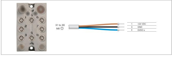
X67CA0D40.xxxx: M8 straight sensor cable X67CA0D50.xxxx: M8 angled sensor cable
