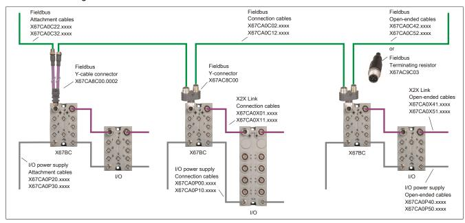
The bus terminating resistor is housed in a connector and screwed onto the Y-connector when needed.
