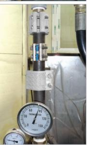
80°C×30min.×20kg/cm<sup>2</sup> Hightemperature circulation test
