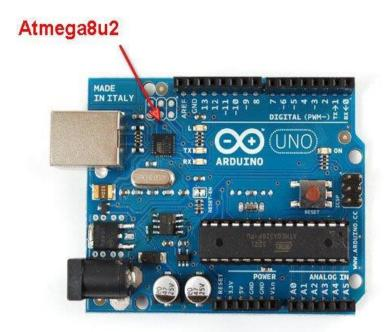
The Uno has changed that by exchanging the FT232RL chip with an atmega8u2 chip. There are a few things that are possible with this new chip but before we discuss that lets make it clear that by default, this chip acts identically to the FTDI chip that it replaces. It's just a USB-serial port!
