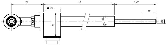
Model SM260 ..GK (IP67 with ball joint and Pg9-fastener with cable 3x 0.56mm<sup>2</sup>)
