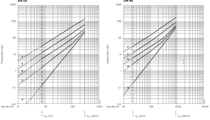
For a pressure drop of more than 1 bar, it is recommended to use the next larger meter size. Maximum permissible pressure drop = 3 bar
