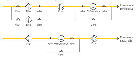
If the flow meter is installed on the suction side of the pump, the pressure drop at the max. allowed flow rate and highest possible viscosity must be taken into account. Also to be considered are installed filters.
