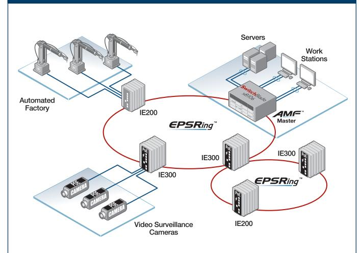
EPSRing<sup>™</sup> and ITU-T G.8032 provide high speed resilient ring connectivity. This diagram shows the IE Series in a double ring network topology.
