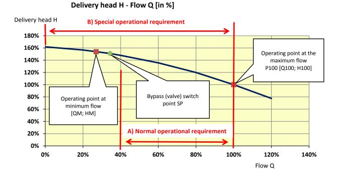
Figure 7 Normal and special operational requirement
