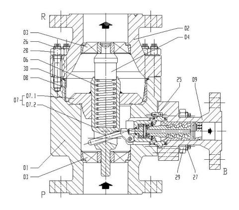
Description Item 01 Lower body 02 Upper body 03 Valve stemguide 04 Guide bolt 06 Spring 07 Non-return plug assembly 07.1 Non-return plug 07.2 Stem 80 Liner or venturi ring 09 Bypass branch 25 Guide Pin 26 Stud bolt 27 Stud bolt 28 Hexagon Nut 29 Hexagon Nut 30 O-ring
