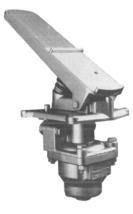
The H-1 CONTROLAIR Valve is a pedal actuated, 3-way pressure regulating valve, suitable for applications where the valve portion extends below the floor level. Depressing the pedal increases the outlet pressure. The pedal is selfreturning. This valve is suitable for brake and clutch control or any use where foot operation pressure control is desired. Approx. weight:8½ lbs. (3.9 Kg)
