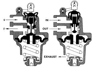
INCREASING PRESSURE DECREASING PRESSURE When the CONTROLAIR Valve is in decreasing pressure position, the inlet valve is closed and the exhaust valve is open to vent the OUT pressure to atmosphere, inlet pressure is on top of the closed inlet valve.
