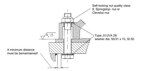
After the first 50 hours of operation the unbalance vibrator, the fixing screws must be retightened to the correct tightening torque.
