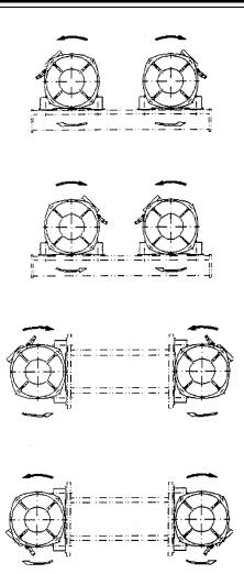
Before starting up the vibrating machine the correct **<u>opposed</u>** direction of rotation of the unbalanced mass vibration generators must be checked, as follows:
