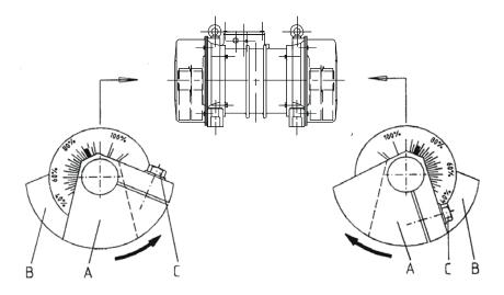
On both sides of the unbalanced mass vibration generator the centrifugal weights should be set to the required value (which can be read off on the % scale). The set values must be the same on both sides.
