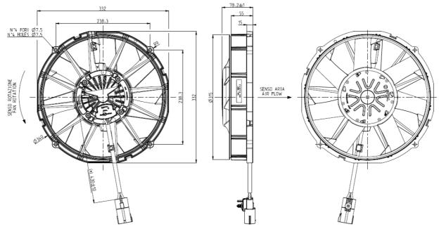
Fixing recommendation: use M6 bolts for fixing. Nominal tightening torque 3 +1/0 Nm Nominal torque defined for brand new, clean and lubricant-free bolts.
