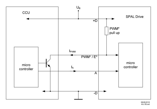
The CCU electronics and the Drive electronics are connected via two unidirectional lines.
