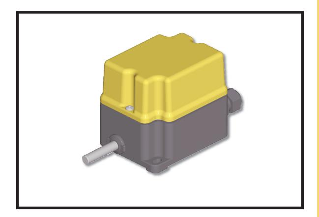
■ The rotary limit switch is used to control the movement of industrial machinery. It operates as an auxiliary controller of electrical motors through a power interface, such as a contactor or PLC. Suitable for heavy duty, its shaft is connected to the motor and, after a set number of revolutions, the cams operate the switches, thus starting the predetermined movement.
