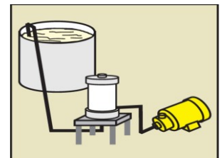
SOLUTION TRANSFER w/PRIMING CHAMBER
