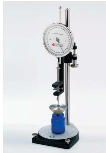
K19500 Penetrometer with K20800 Penetration Cone
