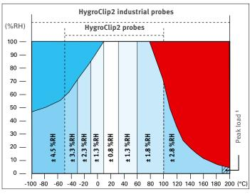
$<sup>^{1}</sup>$  The peak load at 200 °C is for a period of 100 hours; 190 °C constant load. See the sensor data sheet for detailed information on the chemical pollution loads for the sensor.
