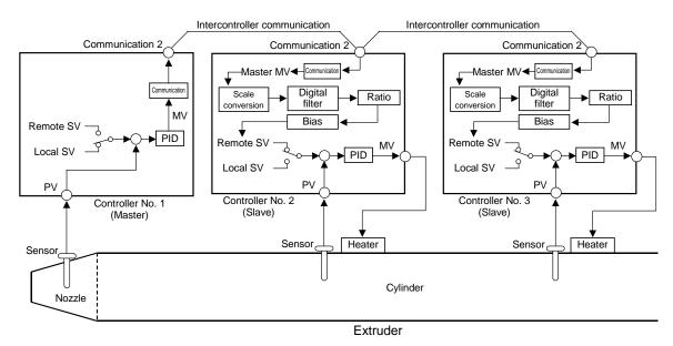
Block diagram of Cascade control by Intercontroller communication
