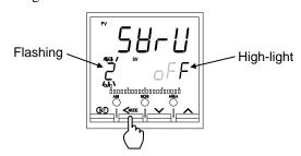
**14.** Set the Memory area 3 Setting change rate limiter, Area soak time, and Link area number by the same procedures as described in steps **3** to **9** (P. 6-56).
