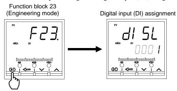
Set the Digital input (DI) assignment by pressing the UP or DOWN keys.
