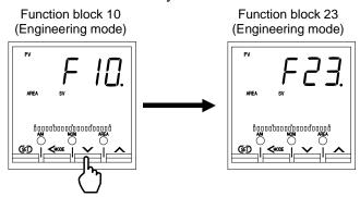
4. Press the SET key to change the Digital input (DI) assignment screen.
