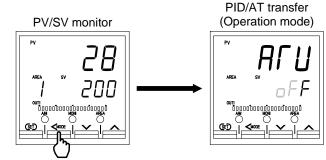
Press and hold the Shift key for 2 seconds
