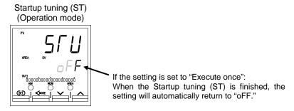
When Startup tuning (ST) was interrupted, the setting does not change to "oFF." Startup tuning (ST) starts when the restart conditions are satisfied.
