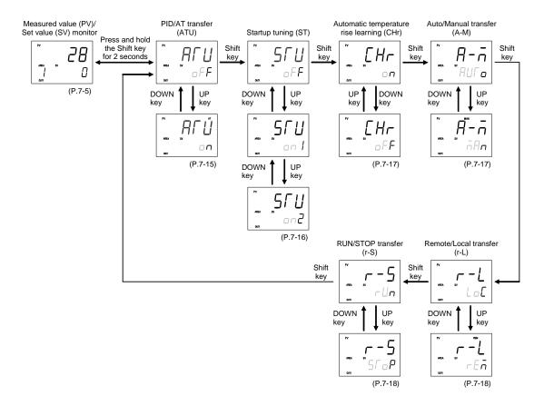
Transferring the Operation mode immediately performs control in the mode transferred.
