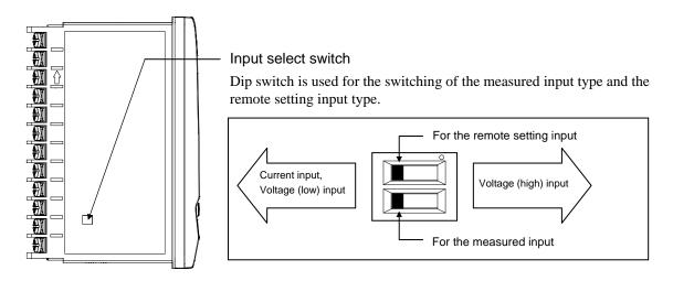
To change the input type, refer to **Input type** (**P. 7-69**), **Remote setting input type** (**P. 7-77**) in the Engineering mode.
