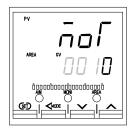
Set the Control motor time required for rotation from the fully closed position to the fully opened position.
