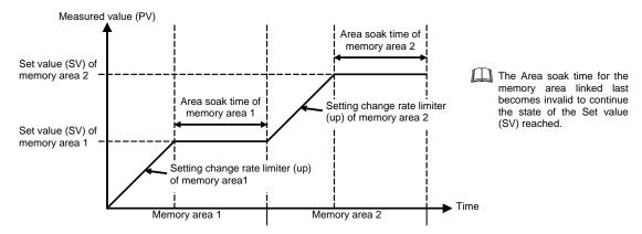
Time required while the Setting change rate limiter is being operated is not included in the Area soak time.
