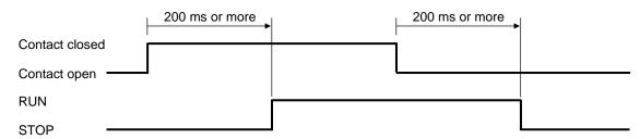
After the contact is transferred, it takes "200 ms + 1 sampling cycle\*" until the action of this instrument is actually selected.
