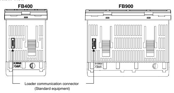
Use our communication converter COM-K (sold separately) to connect FB400/900 Series and personal computer. Then, the cable (cable length: 1.5 meters) for connection between FB400/900 series and our communication converter COM-K is optional.
