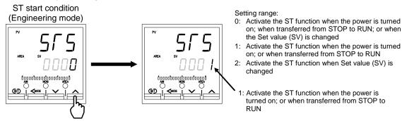
**6.** Press the SET key to store the new value. The screen goes to the ST proportional band adjusting factor screen.
