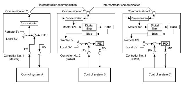
Block diagram of Ratio setting by Intercontroller communication
