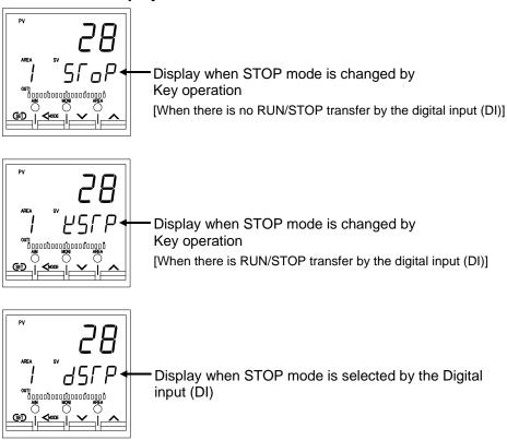
The display unit to display the STOP character can be changed from the SV display section to the PV display section by referring to "STOP display" in the Engineering mode.
