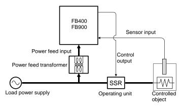
The Power feed forward function is used together with the Output change rate limiter function, the Manipulated output value may exceed the limit of the Output change rate limiter.
