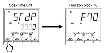
**9.** To return the PV/SV monitor, press the MONI key (for direct key type 1), or press the Shift key while pressing the SET key.
