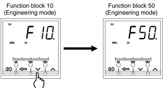
4. Press the SET key until External input type setting screen is displayed.
