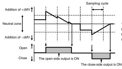
The controller does not output the  $\Delta MV$  to a control motor when the PID computed output value is within the neutral zone.
