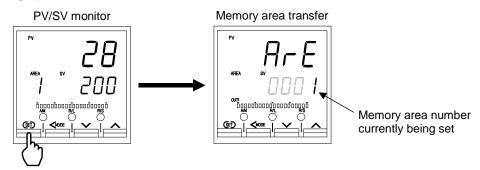
2. Select the memory area number which needs to be changed by pressing the UP or DOWN key.
