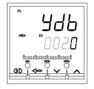
Set the output OFF zone between open-side and close-side outputs.
