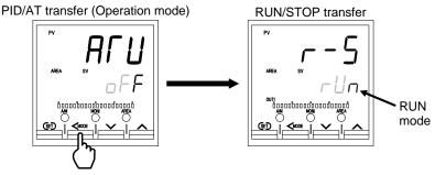
3. Pressing the UP key changes to STOP mode from RUN mode.
