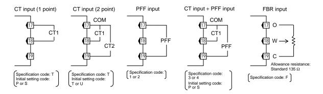
• Current transformer (CT) input, Power feed forward (PFF) input, and Feedback resistance (FBR) input are not isolated between Measured input.
