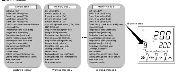
In addition, it is possible to perform Ramp/Soak control by linking each memory area. It is possible to perform Ramp/Soak control of up to 16 segments (8 steps).
