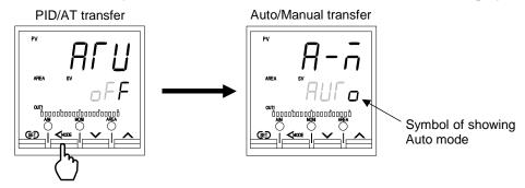
**3.** Press the UP key to change to the Manual mode from the Auto mode. The Manual (MAN) mode lamp lights.
