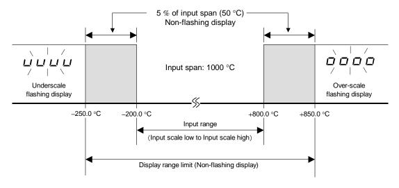
However, if the Input error determination point (low) or the Input error determination point (high) is set within the input range, up to  $\pm 5$  % of input span from the Input error determination point (low) or (high) becomes the PV flashing display range.
