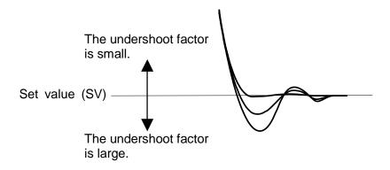
If the Undershoot suppression factor is set too small, the undershoot function acts excessively and prevents the Measured value (PV) from reaching the Set value (SV). As a result, the PV stabilizes at an offset or approaches the set value very slowly, preventing normal control. In this event, change the setting for the Undershoot suppression factor to a slightly higher value.
