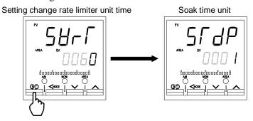
7. Select the Area soak time unit which needs to be changed by pressing the UP or DOWN key. If unnecessary to be changed, use their factory set values.
