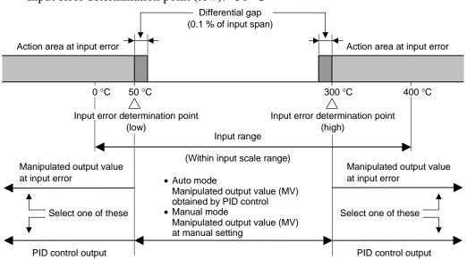
[Manipulated output action at input error]
