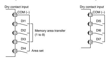
• Digital input from external devices or equipment should be dry contact input. If it is not dry contact input, the input should have meet the specifications below.
