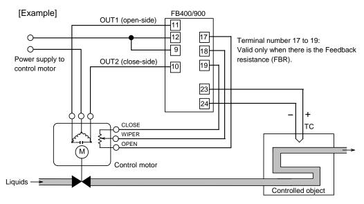
The details of setting differ depending on the presence or absence of Feedback resistance (FBR) input.
