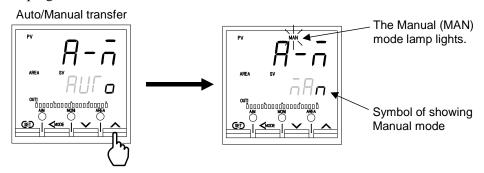
• To change from the Manual mode to the Auto mode, press the DOWN key.
