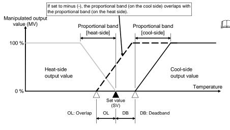
The diagram is an example when setting 0.0 to the Overlap/Deadband reference point.
