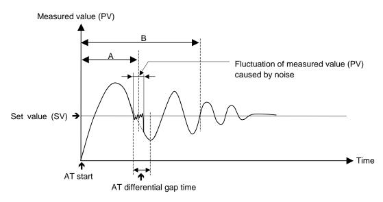
The factory set value of the AT cycle is 2 cycles.
