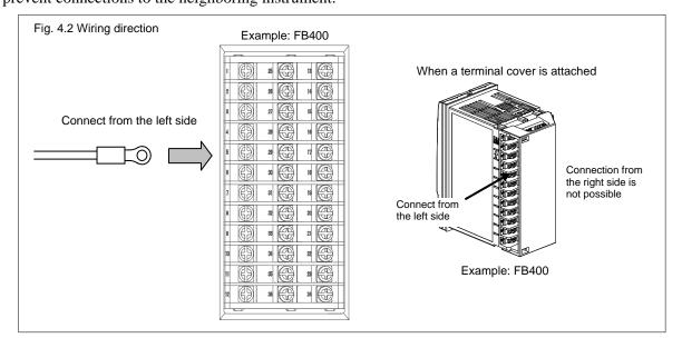
• Up to two solderless terminal lugs can be connected to one terminal screw. However, in this case, reinforced insulation cannot be used.
