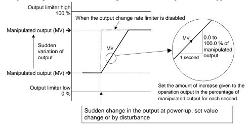
The output changes at specific rates set by Output change rate limiter (up) even under the situations where a sudden output change would occur without Output change rate limiter function. There is also independent Output change rate limiter (down).
