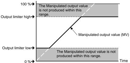
Output limiter is available for ON/OFF action.
