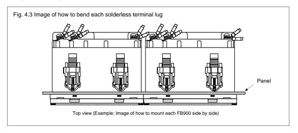
If solderless terminal lugs other than those in not specified dimensions are used, terminal screws may not be tightened. In such a case, bend each solderless terminal lug in advance and then conduct wiring. If the terminal screw is forcibly tightened, it may be damaged.
