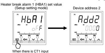
**3.** Set the address by pressing the UP or DOWN keys. Setting range: 0 to 31 (Factory set value: 0)
