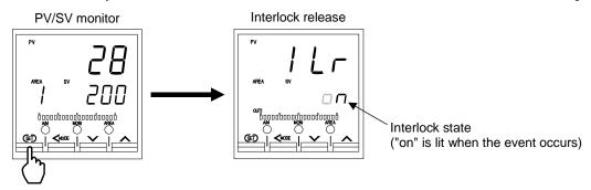
2. Press the DOWN key to release the interlock.
