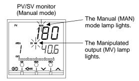
2. Set the Manipulated output value (MV) by UP or DOWN keys.
