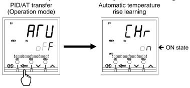
3. When the UP key is pressed, it switches from "oFF" to "on." In addition, since the shipping value is "on," when executing Automatic temperature rise leaning, it can be used as is.
