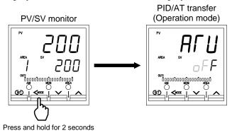
2. If set to "on" by pressing the UP key, the Autotuning (AT) function starts. At this time, the AT lamp flashes.
