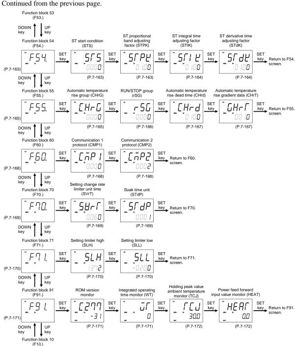
Display returns to the SV setting & monitor mode if no key operation is performed within 1 minute (except during the Feedback adjustment or the Power feed forward input value monitor display).
