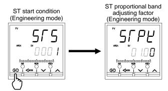
7. To return the PV/SV monitor, press the MONI key (for direct key type 1), or press the Shift key while pressing the SET key.
