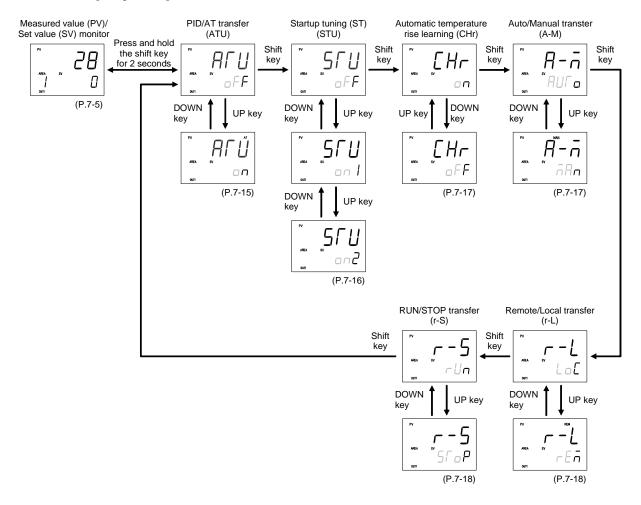
The SET key as well as the shift key enables the transfer of operation items.
