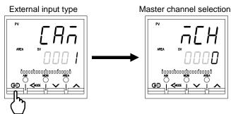
7. Press the UP key or DOWN key and set the address (value set by the Device address 2 screen) of the controller specified the cascade control master. Set the Master channel to only the slave controller. No setting of the master controller is required.
