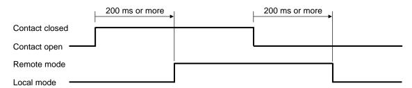
After the contact is transferred, it takes "200 ms + 1 sampling cycle<sup>\*</sup>" until the action of this instrument is actually selected.
