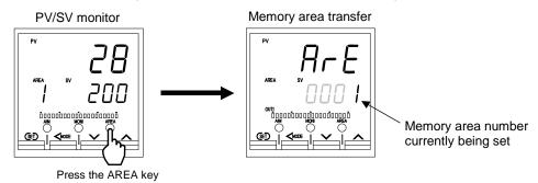
2. Select the memory area number which needs to be changed by pressing the UP or DOWN key.
