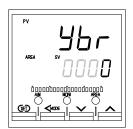
Set the action at Feedback resistance (FBR) input error. Setting range: 0: Depending on the valve action at STOP
