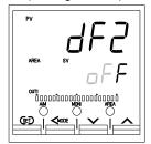
If the External input type is Remote setting input, the Cascade digital filter screen becomes the RS digital filter screen and if Intercontroller communication ratio setting, it becomes the Ratio setting digital filter screen. In other places, this is indicated as "RS digital filter."
