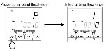
After a new value is displayed on the display by using UP and DOWN keys, if no key operation is performed within 1 minute without pressing SET key, this instrument returns to the PV/SV monitor screen and the Proportional band [heat-side] set value will not be changed.
