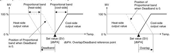
To change Deadband when the Overlap/Deadband reference point is 0.5, the Proportional band on heat-side and cool-side shift equidistantly to the midpoint of the Overlap/Deadband.
