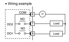
• Output type is only Relay contact output.
