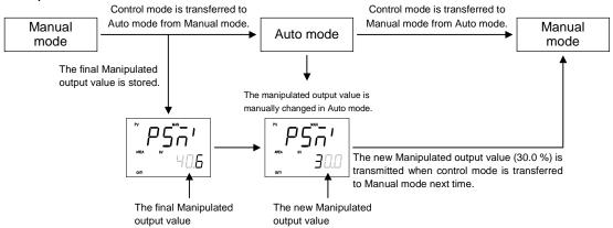
Manipulated output value can be changed by the UP, DOWN or shift keys.
