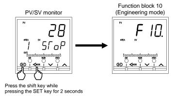
3. Press the UP or DOWN key until Function block 51 screen is displayed.
