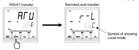
**3.** Press the UP key to change to the Remote mode from the Local mode. The Remote (REM) mode lamp lights.
