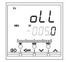
Set the low-limit value of the valve position.
