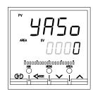
Set to maintain ON state for the close-side (or open-side) output when the valve position is fully closed (or opened).
