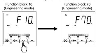
4. Press the SET key to change the screen to the Setting change rate limiter unit time setting screen.
