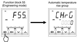
5. Select the Automatic temperature rise group number which needs to be changed by pressing the UP or DOWN key.
