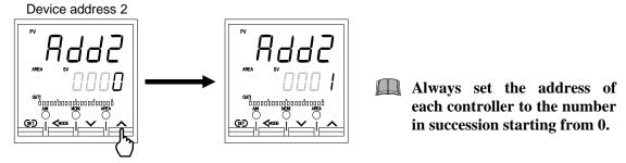
After a new value is displayed on the display by using UP and DOWN keys, if no key operation is performed within 1 minute without pressing SET key, this instrument returns to the PV/SV monitor screen and the address will not be changed.
