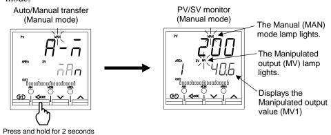
When in STOP mode, no Manual (MAN) mode lamp turns on.
