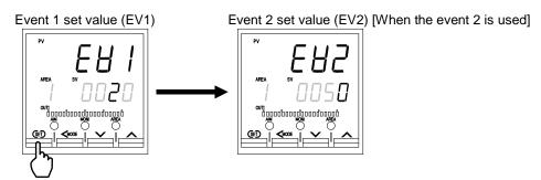
After a new value is displayed on the display by using UP and DOWN keys, if no key operation is performed within 1 minute without pressing SET key, this instrument returns to the PV/SV monitor screen and the Event 1 set value (EV1) will not be changed.
