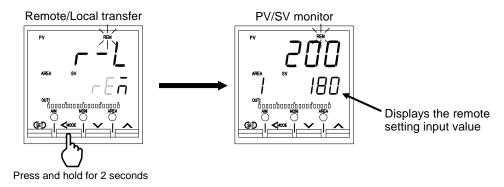
When in STOP mode, no Remote (REM) mode lamp turns on.
