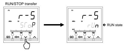
For the RUN/STOP transfer, refer to **6.4 RUN/STOP Transfer** (**P. 6-11**). For the group RUN/STOP, refer to **6.14.3 Group RUN/STOP function** (**P. 6-63**).
