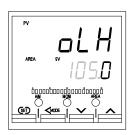
Set the high-limit value of the valve position. Setting range: Output limiter low (MV1) to +105.0 % (Factory set value: 105.0)
