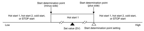
Start determination point setting is conducted in Engineering mode. For details, refer to **7.5 Engineering Mode (P. 7-124)**.
