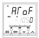
Set the lower limit values of the valve position (Feedback resistance input) which is opened and closed by output ON/OFF at Autotuning (AT) execution.
