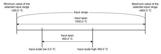
When the scale for temperature input is changed, it is recommended to be changed within the input range. If any value exceeding the input range is set, input resolution may vary.
