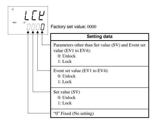
In the Set lock level, data lock is not possible for following parameters.
