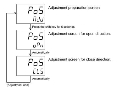
Display returns to the PV/SV monitor screen if no key operation is performed within 1 minute (except during the feedback adjustment).
