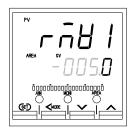
Set the valve position at control STOP. Setting range: -5.0 to +105.0 % (Factory set value: -5.0)
