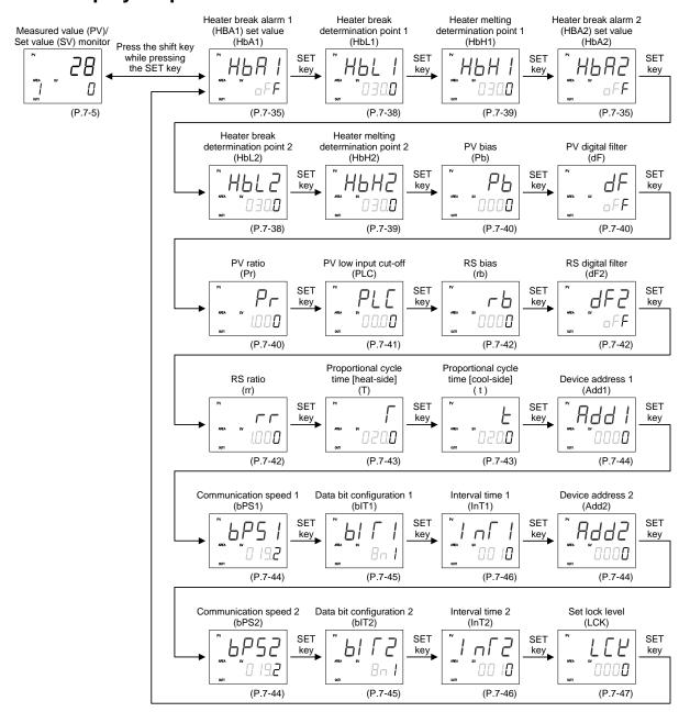
Some parameters may not be displayed when the relevant function is not set so as to be activated or no relevant specification is selected when ordering.
