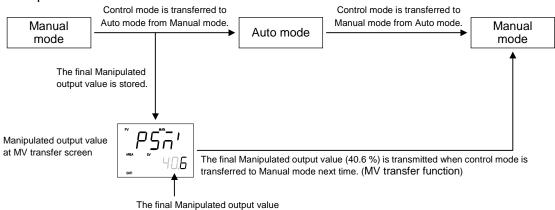
In addition, on this screen it is possible to manually change Manipulated output values (MV1 and MV2) in Auto mode. However, it they are changed in Auto mode, these manipulated output values thus changed are transferred when selected to the Manual mode next time.
