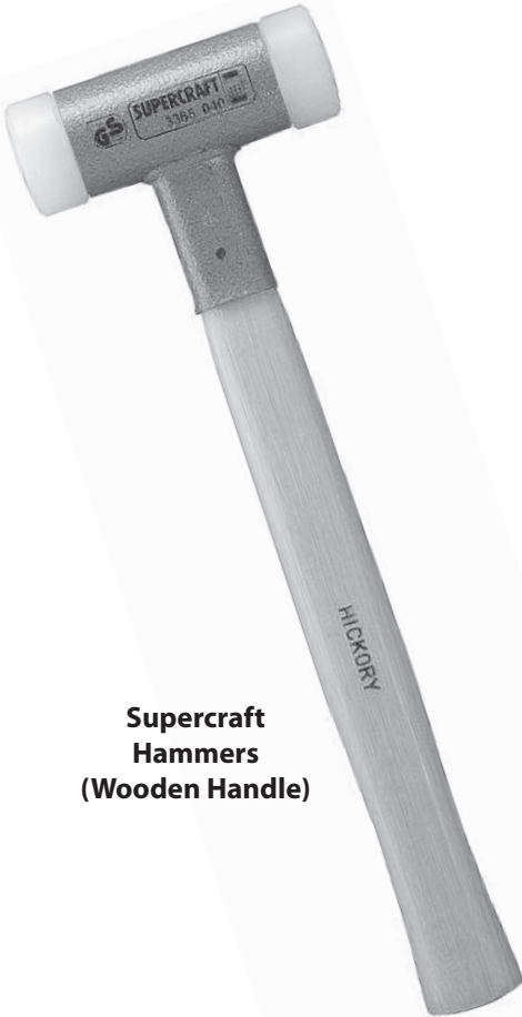
No-Rebound Hammers are filled with special steel pellets that transfer momentum to the impact point.
