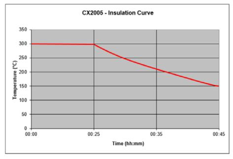
Tested in combination with the Insulation Box CX2005 and **Insulation Box Logger Bracket CX3050** with a start temperature of 20°C (68°F). (So without heat absorber)
