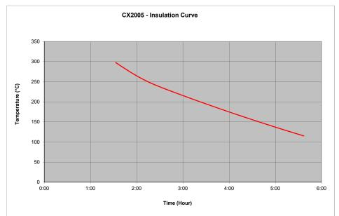
Tested with the **insulation box CX2005** in combination with the **energy absorber CX2011** (a high density energy-collecting media) with a start temperature of 20°C (68°F).
