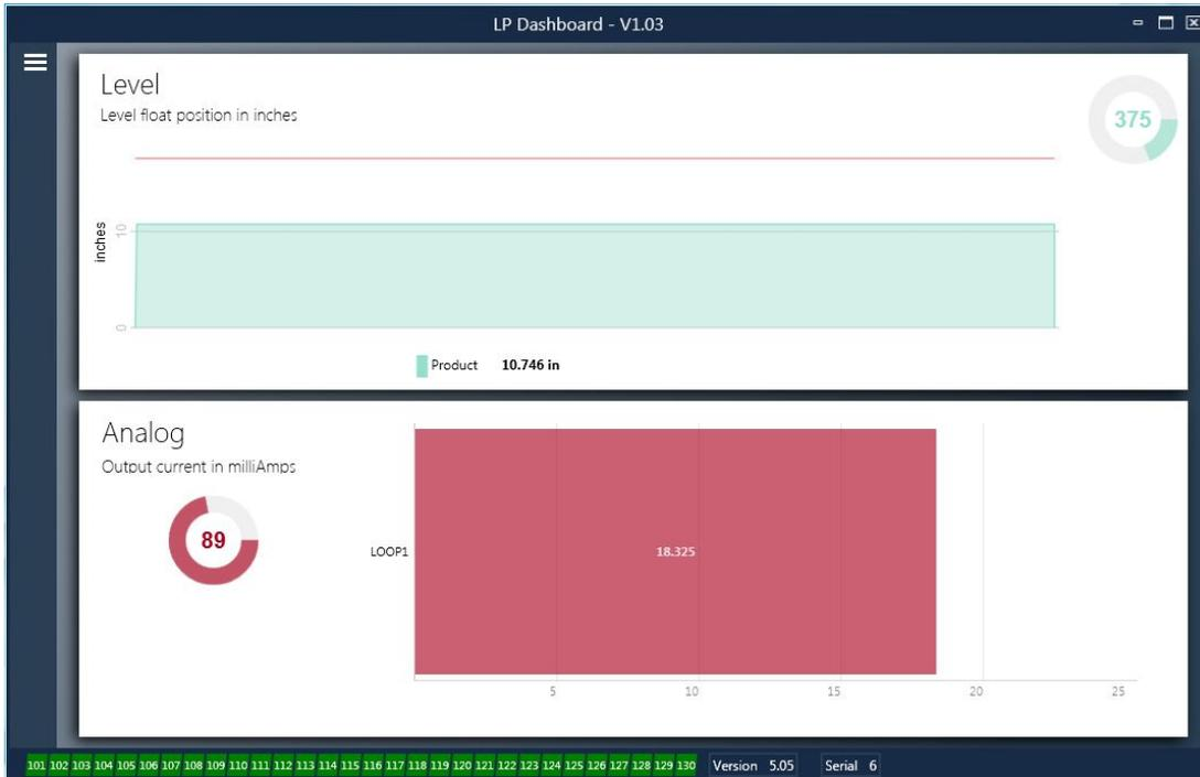
The level panel on top shows the level measurement for the Product level. The bold numbers are the numerical level and the graph is a time lapse of the graphical representation of the numbers. The red line is the approximate maximum level based off of the order length of the level transmitter. The numbers on the top right of the level panel are the Trigger Level for the product float. These are a representation of how strong of a return signal the level transmitter is experiencing.
