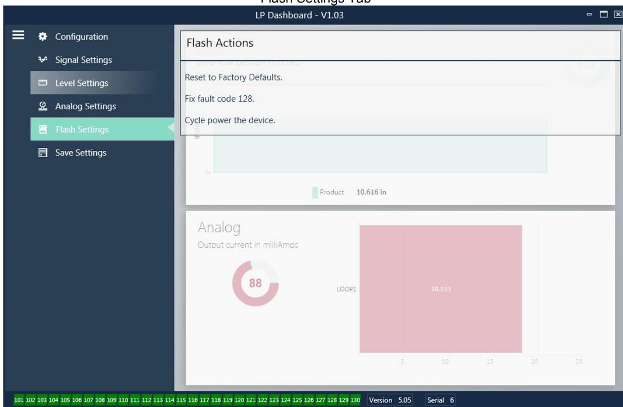
**Reset to Factory Defaults:** Allows the end user to reset all settings back to the original settings as they were when they left the factory. This is intended to be used as a first step in trouble shooting. Do note, the Zero and Span set points will reset to factory settings.
