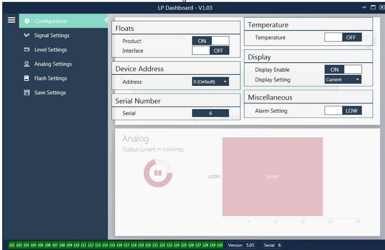
The Configuration tab allows the level transmitter to be configured for the specific application.
